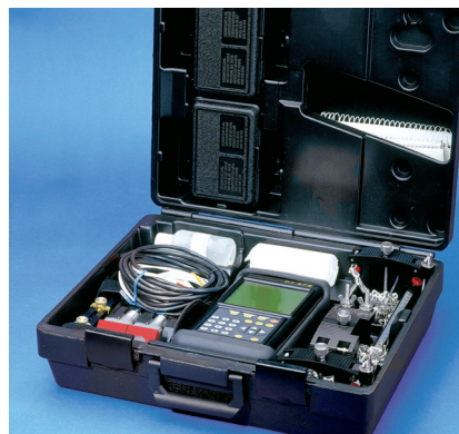
The complete TransPort flowmeter system fits in a compact carrying case.
